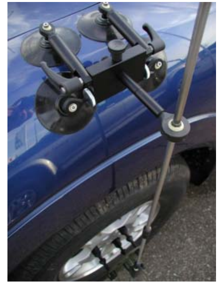
Holding Plate with 4 Suction Cups and lengthened Slip Joint
