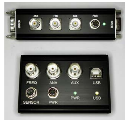
SB2 and SB3 Interconnection Box
