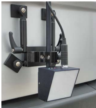
GSS14 with magnetic holder on the tailgate of a van.
