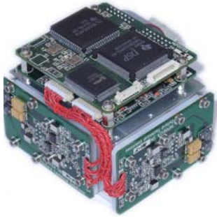
Inertial Sensors in the RT2000 product family include servo-grade accelerometers and precision MEMS angular rate sensors. Powerful 40MHz floating point DSP takes care of coning, sculling and aliasing.
