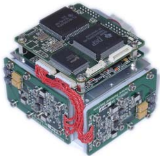
Inertial Sensors in RT4000 include servo-grade accelerometers and precision MEMS angular rate sensors. Powerful 40MHz floating point DSP takes care of coning, sculling and aliasing.
